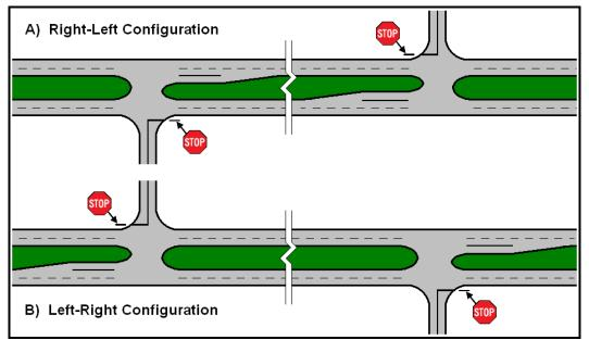
FIGURE 51. Offset T-intersection conceptual schematics
