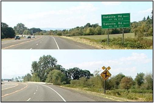
FIGURE 57. Offset T-intersection signage at OR-34 & Oakville Road
