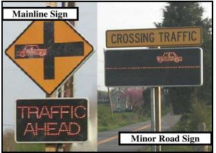
FIGURE 107. Collision Countermeasure System tested in Virginia (79)
