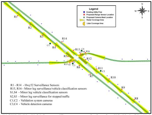
FIGURE 70. Vehicle surveillance system deployed at US-52 & CSAH-9
