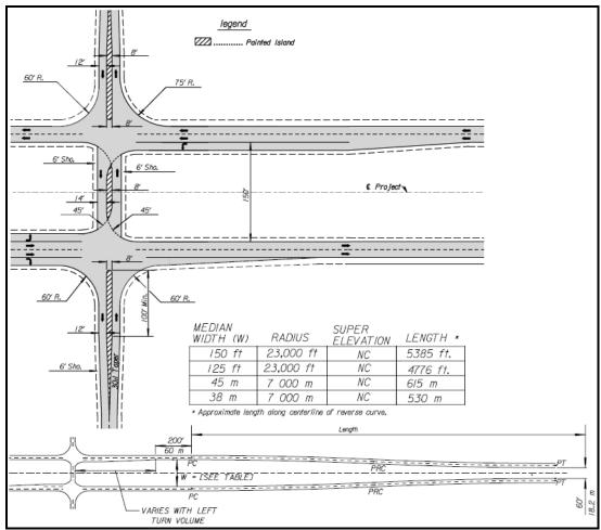
FIGURE 24. KDOT standard plan for wide median intersection (36)
