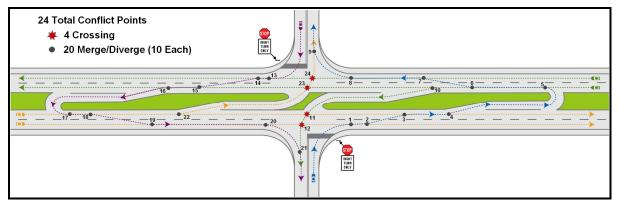
FIGURE 32. J-turn intersection schematic & conflict point diagram
