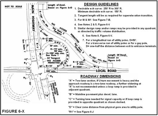
FIGURE 65. NJDOT design standard for far-side jughandle intersection (68)
