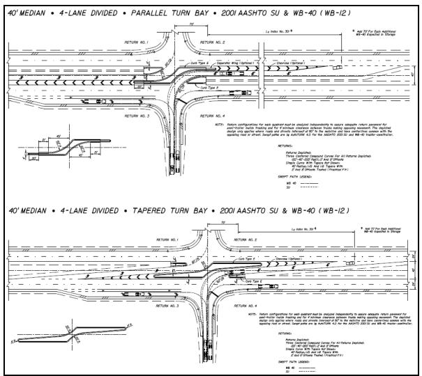
FIGURE 38. FDOT standard plans for directional median openings (54)
