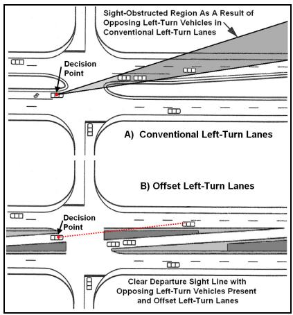
FIGURE 87. Offset left-turn lane design concept illustration
