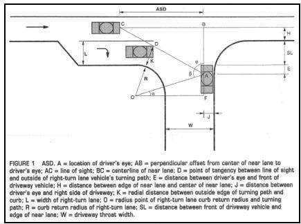
FIGURE 82. Minimum right-turn offset calculation trigonometry diagram (86)
