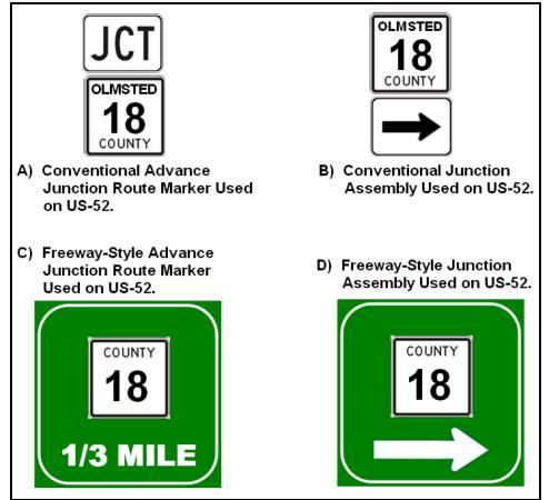
FIGURE 105. Example of intersection guide signing along US-52 (before & after)
