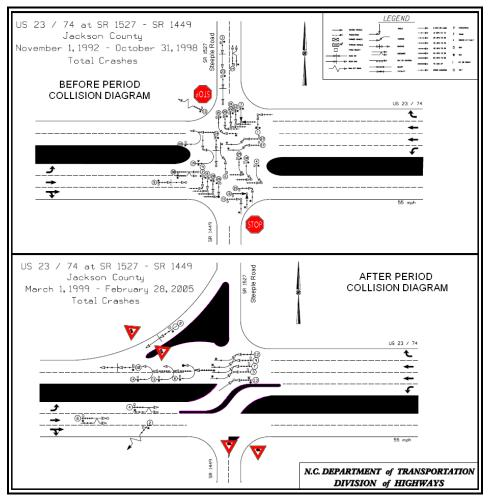
FIGURE 46. Before and after collision diagrams at US-23/74 & SR-1527/1449 (59)
