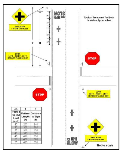
FIGURE 71. Plan view of static gap assistance markings deployed by PennDOT (82)
