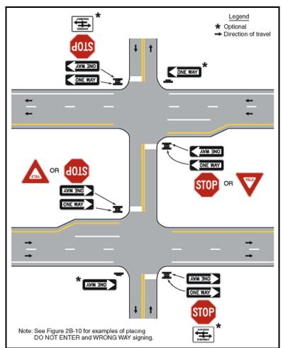
FIGURE 25. MUTCD Figure 2B-13; example of ONE WAY signing for divided highways with medians of 30 feet or greater (31)
