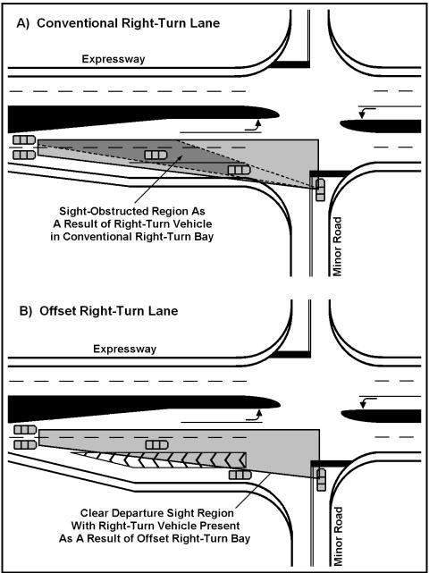
FIGURE 80. Offset right-turn lane design concept illustration
