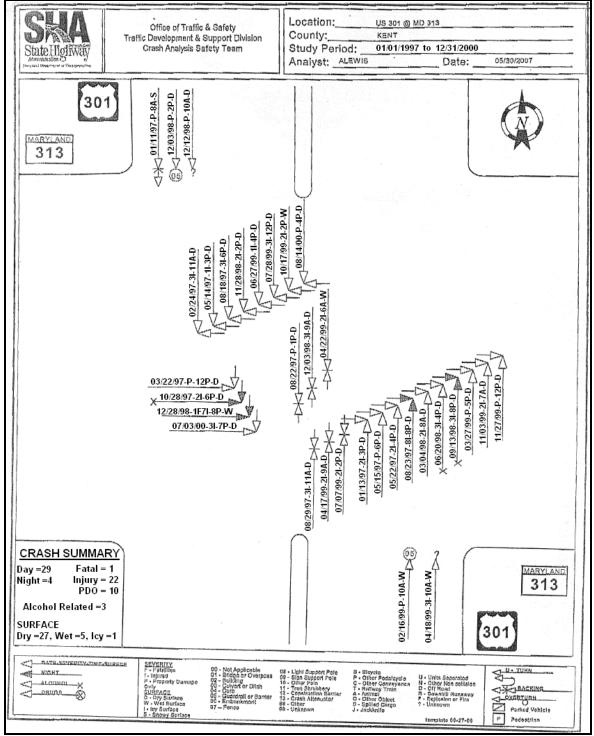
FIGURE 41. Collision diagram at US-301 & MD-313 before J-turn construction (57)
