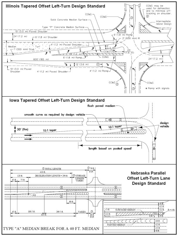
FIGURE 96. Offset left-turn lane designs in Illinois, Iowa, and Nebraska (7, 85, 91)
