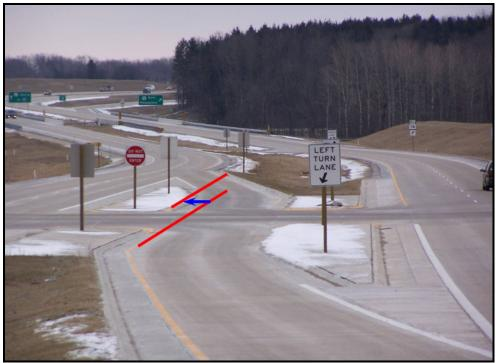
FIGURE 94. Offset left-turn lanes designed with a negative offset (incorrect design)
