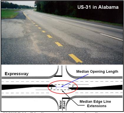
FIGURE 23. Edge line extensions through median crossover
