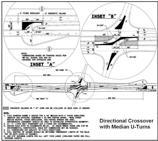
FIGURE 35. NCDOT standard plan for J-turn intersection (53)
