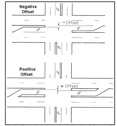
FIGURE 90. Illustration of negative and positive left-turn offsets (90)
