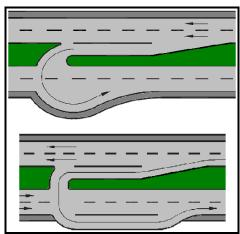
FIGURE 33. Examples of U-turn median openings with left-turn lanes & loons
