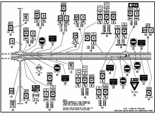
FIGURE 37. MoDOT standard signing plan for J-turn intersection (37)
