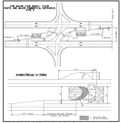
FIGURE 36. MoDOT standard plan for J-turn intersection (37)
