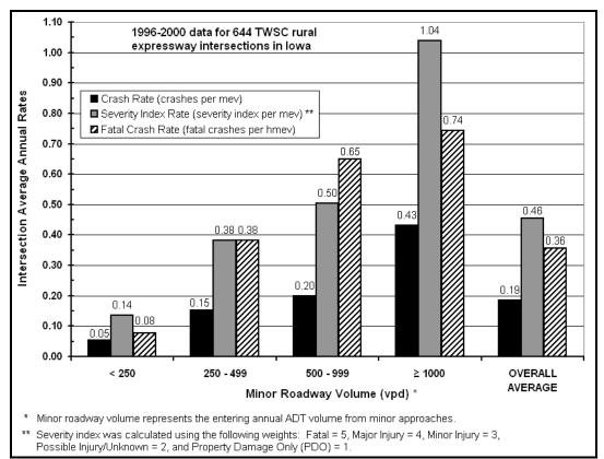
FIGURE 5. Intersection crash rates & severity by minor road entering volume (2)
