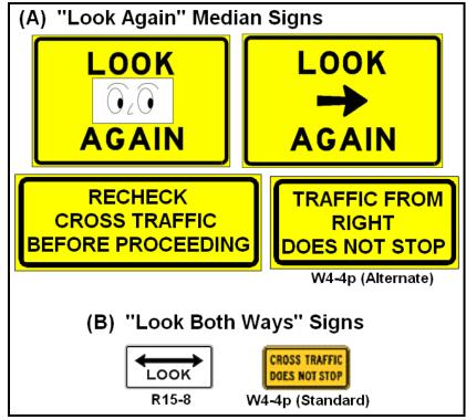
FIGURE 27. Warning signs used to prevent right-angle collisions
