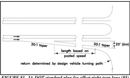
FIGURE 81. IA-DOT standard plan for offset right-turn lane (85)
