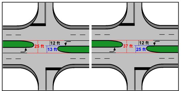
FIGURE 21. Expressway intersection median width/storage illustration
