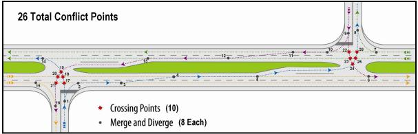
FIGURE 52. Conflict point diagram for an offset T-intersection
