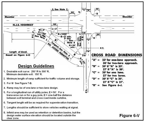
FIGURE 64. NJDOT design standard for near-side jughandle intersection (68)
