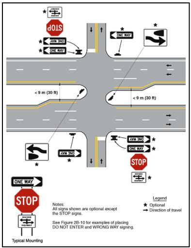
FIGURE 26. MUTCD Figure 2B-14; example of ONE WAY signing for divided highways with medians less than 30 feet (31)
