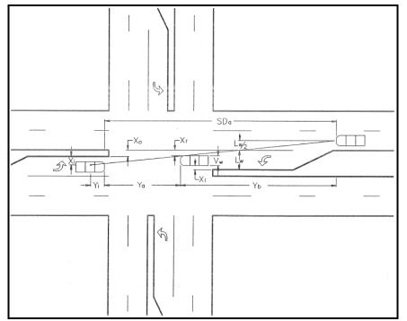
FIGURE 91. Minimum left-turn lane offset calculation trigonometry (90)
